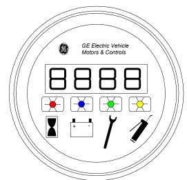
The GE Standard Dash Display is a four segment Light Emitting Diode (LED) instrument that displays the GE LX, ZX, and SX Status Codes, Hourmeter Readings, Battery Discharge Indication, and Maintenance Required Code. The four LED's above the symbols indicate the active readout mode.
